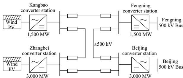
**Fig. 3 Schematic diagram of the structure of the Zhangbei VSC-based DC grid**
