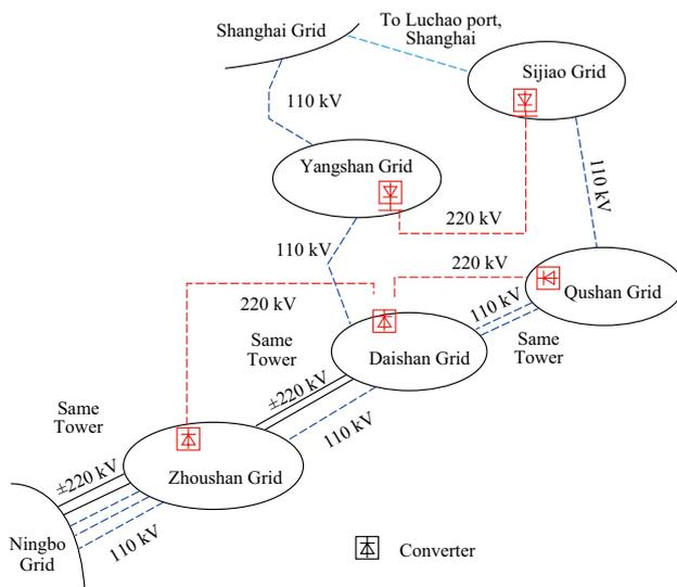
**Fig. 2** Schematic diagram of the structure of the Zhoushan multi-terminal VSC-MTDC project [29]
