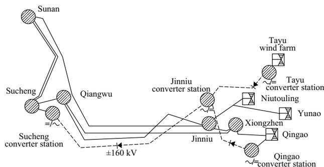
**Fig. 1 Schematic of the structure of the Nan'ao VSC-MTDC project [19]**
