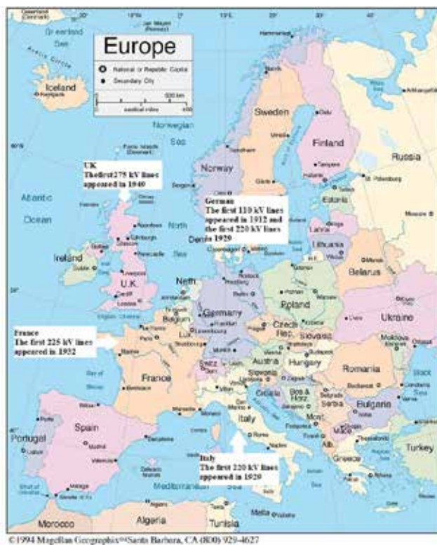
Fig. 2 The update process of transmission voltage in Europe from the early to mid-20th centuries
